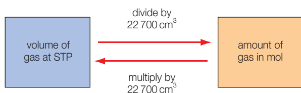
Figure 1.16 Summary of interconversions between the amount of gas and volume (at STP)
