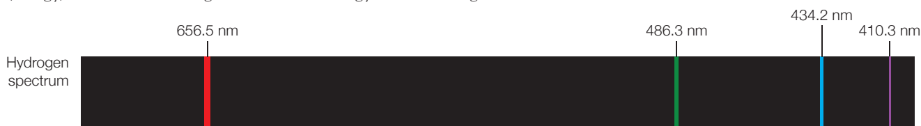
Figure 2.14 The Balmer series: the line spectrum in the visible region for the atomic emission spectrum of hydrogen
